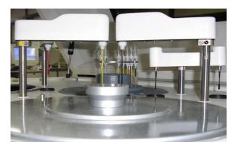
The EM 360's special capacitance probes provide liquid level sensing & separate probes (seen above) ensure reliability of throughput at 360 tests/hour even when the analysis involves double reagents system.
